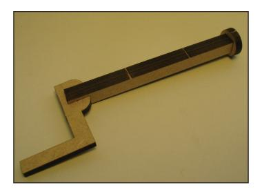
Once dry, chamfer the end slightly so it will be easier to slide the cams and spacers onto the shaft
