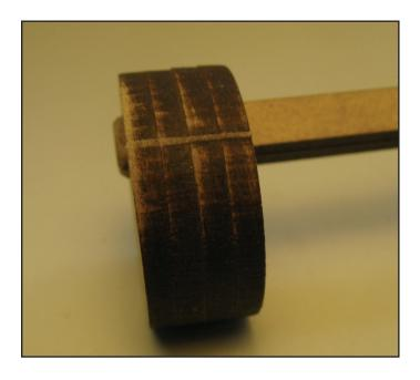
Slide two spacers on the shaft and sand them smooth. These will be at each end of the camshaft and will be turning in the bearing holes in the lifter frame. Check they are a loose fit in the holes.
