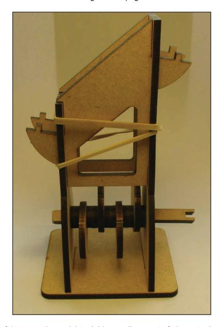
Centre the camshaft between the uprights. Add a small amount of glue onto the shafts near to where they exit from the uprights. Slide the retaining disc in place. Ensure that a bit of sideways movement of the camshaft is still possible. About 1mm is right. Glue the crank handle in place.
