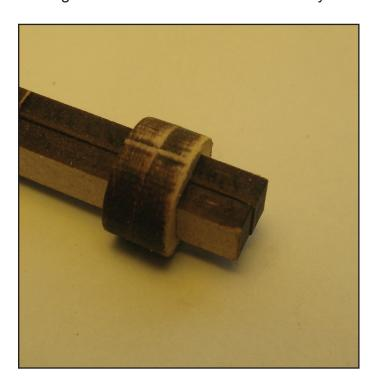
Now onto the camshaft assembly. Slide two spacers onto the shaft so the align with the pip mark towards the end of the shaft that has the cut-our for the crank handle.
