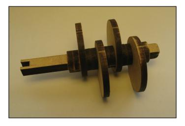
Slide the spacers at each end out, apply a small drop of glue onto the shaft between the spacers and slide them back in place again.
