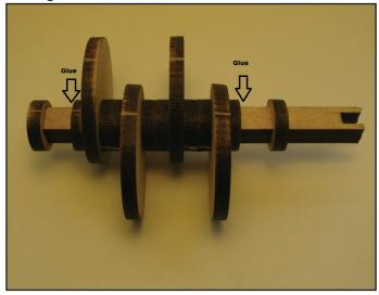
Push firmly on the ends of the spacers so the cams are not wriggling around on the shaft. Leave to dry.
