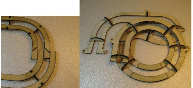
Glue the end doublers onto the zig-zag track pieces. These go on the side of the sheet marked with an X (opposite side of the spacers!).
