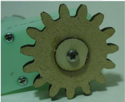
If you find that the mesh with the large gear is a little on the tight side, a spacer or two cut from thin card can be placed under the motor.
