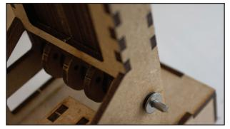
Place a washer on the protruding crankshaft.
